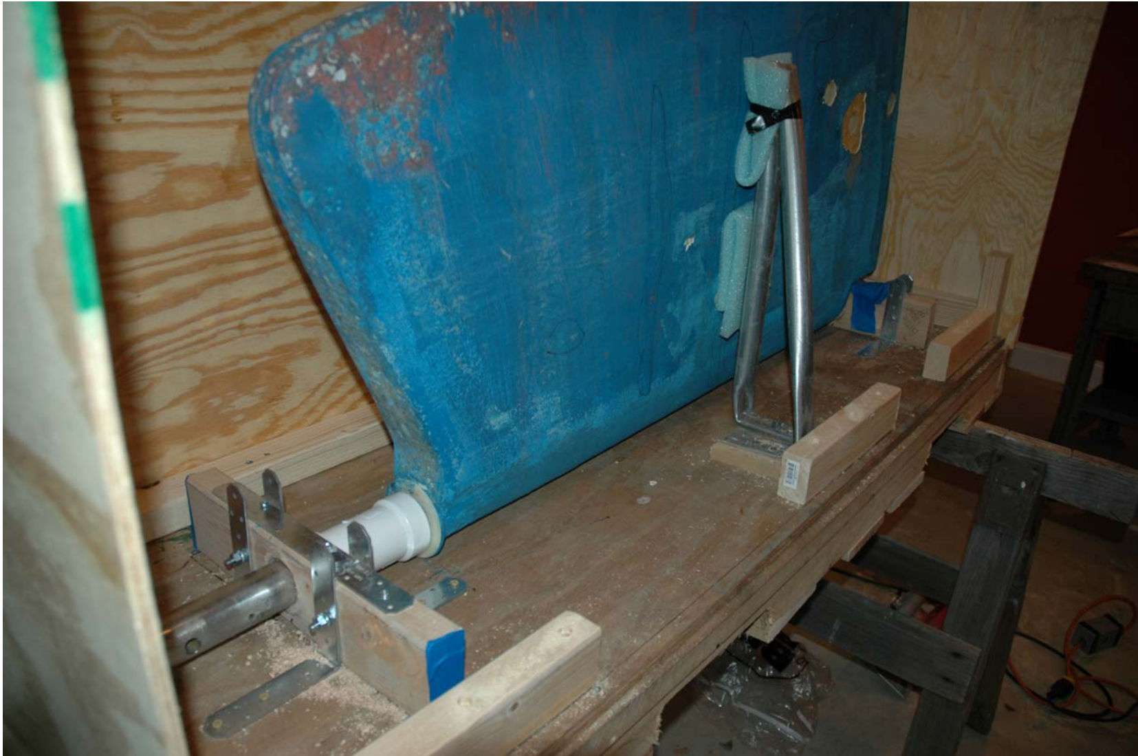
Bracket assemblies support shaft at top and bottom of rudder shaft. Sides supported by brackets and there is a top bracket too.
